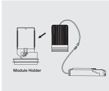
2. Attach module to module holder with spring clip and connect module to driver.
