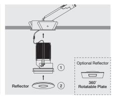
3. Gently insert module holder & reflector from the bottom of the fixture frame.
