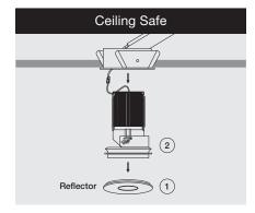
Reverse the installation step 3 for LED module replacement / maintenance.
